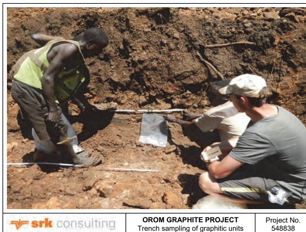
Figure 5-33: Trench sampling of graphitic units
